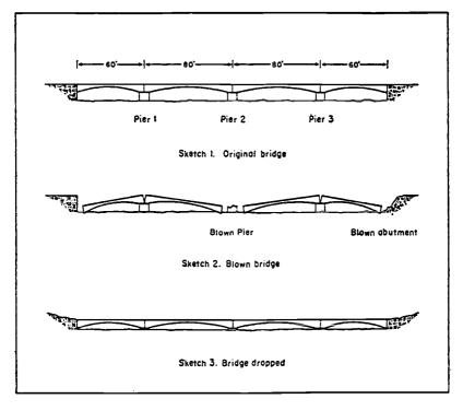
After the site cleared we could see that our calculations were accurate and that the bridge had dropped as planned. The concrete deck of the old bridge now formed a causeway over the banks and stream some four feet above the ground. There was plenty of room underneath for the river to flow at low stage.
